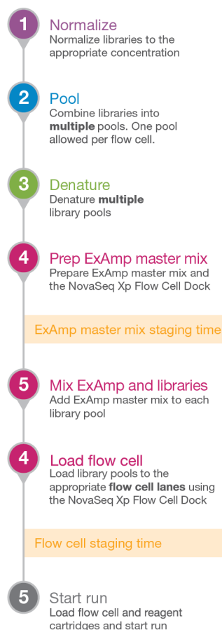
Figure 1: Comparison of NovaSeq Xp and standard workflows —In comparison to the standard workflow, the Xp workflow supports individual lane loading and includes several additional manual touchpoints. These additional steps create staging times (ExAmp master mix staging time and flow cell staging time) that do not exist in the standard workflow and may vary according to automation protocols or user handling.
