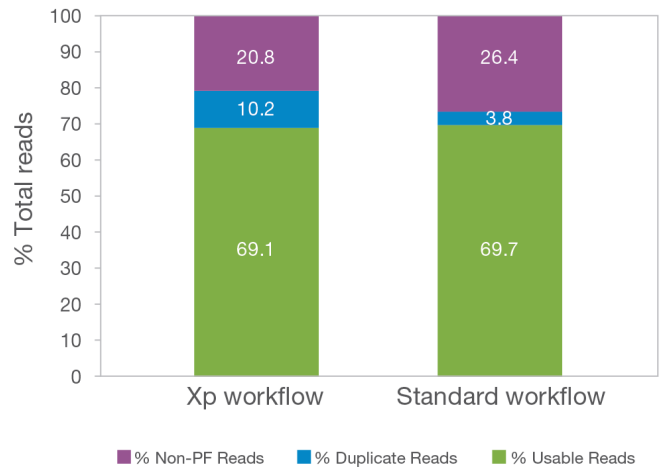
Figure 2: Comparison of NovaSeq standard and Xp workflow sequencing metrics —The Xp workflow data exhibits higher %Duplicate Reads than observed in the standard workflow, while the standard workflow produces higher %Non-PF Reads. Despite these differences, the fraction of Usable Reads remains equivalent between the two workflows.
